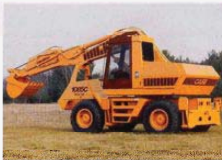
Excavator w/Extendahoe Left side, transport configuration.
