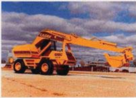
Excavator w/rigid dipper Right side.
